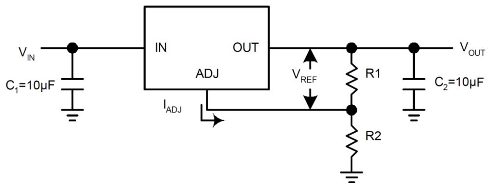
$$V_{OUT} = V_{REF} \times (1 + R2/R1) + I_{ADJ} \times R2$$
